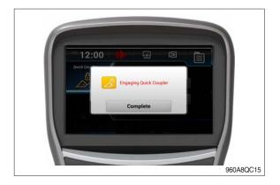
(8) Check whether the quick coupler is locked and touch the 'Complete' button on the monitor screen.
