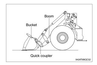
(7) Touch the 'Engage Quick Coupler' button on the monitor screen to lock the quick coupler.
